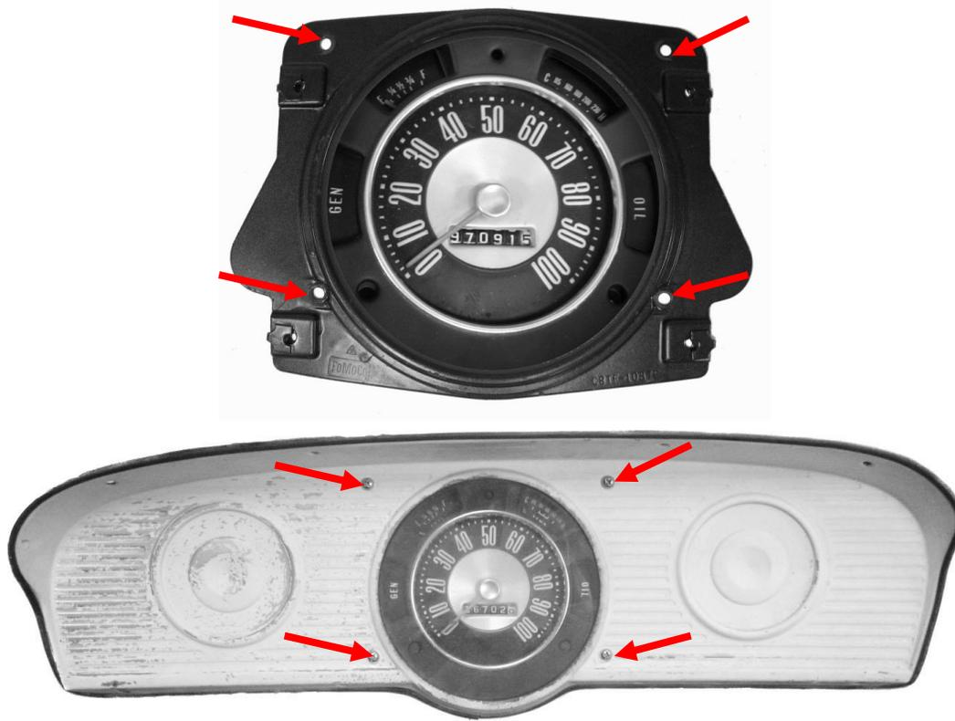
3. The only part that will be re-used is the stamped bezel and the screws that mount the bezel.
